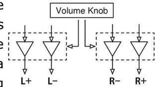
In addition, the TEAC-QVCS provides precise volume control in 0.5dB steps in 'dB' display mode, or 100 steps in 'step' display mode.
