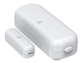
The FOXX Project® Door / Window Sensor is a battery- powered Z-Wave magnetic contact door/ window sensor. The Door / Window Sensor will send radio signals up to 6 associated Z-Wave devices within its own Z-Wave network when the main unit separates from the smaller unit (i.e. the door or window it is attached to is opened).
